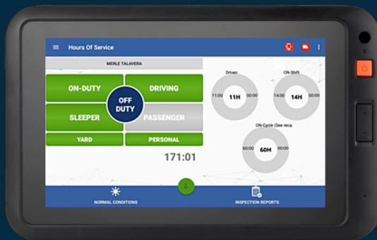
Software is pre-loaded at the factory for faster deployment. The cradle is hardwired directly to your CalAmp LMU-3640 gateway, avoiding connectivity disruptions.
