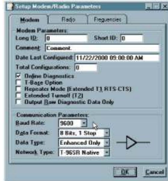
Figure 3b: Serial port parameters selected in the T-96SR Field Programming Software
